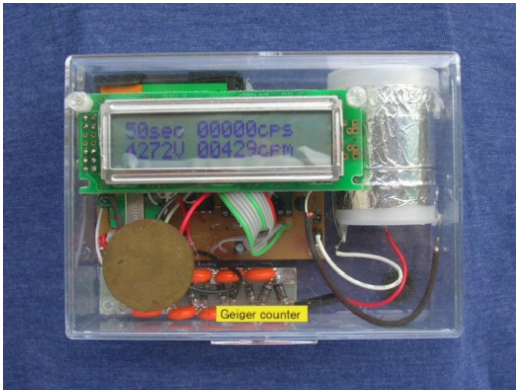
Upper left=Remaining time[sec], Upper right=[cps], Lower left=Operation voltage[V], lower right=[cpm]
